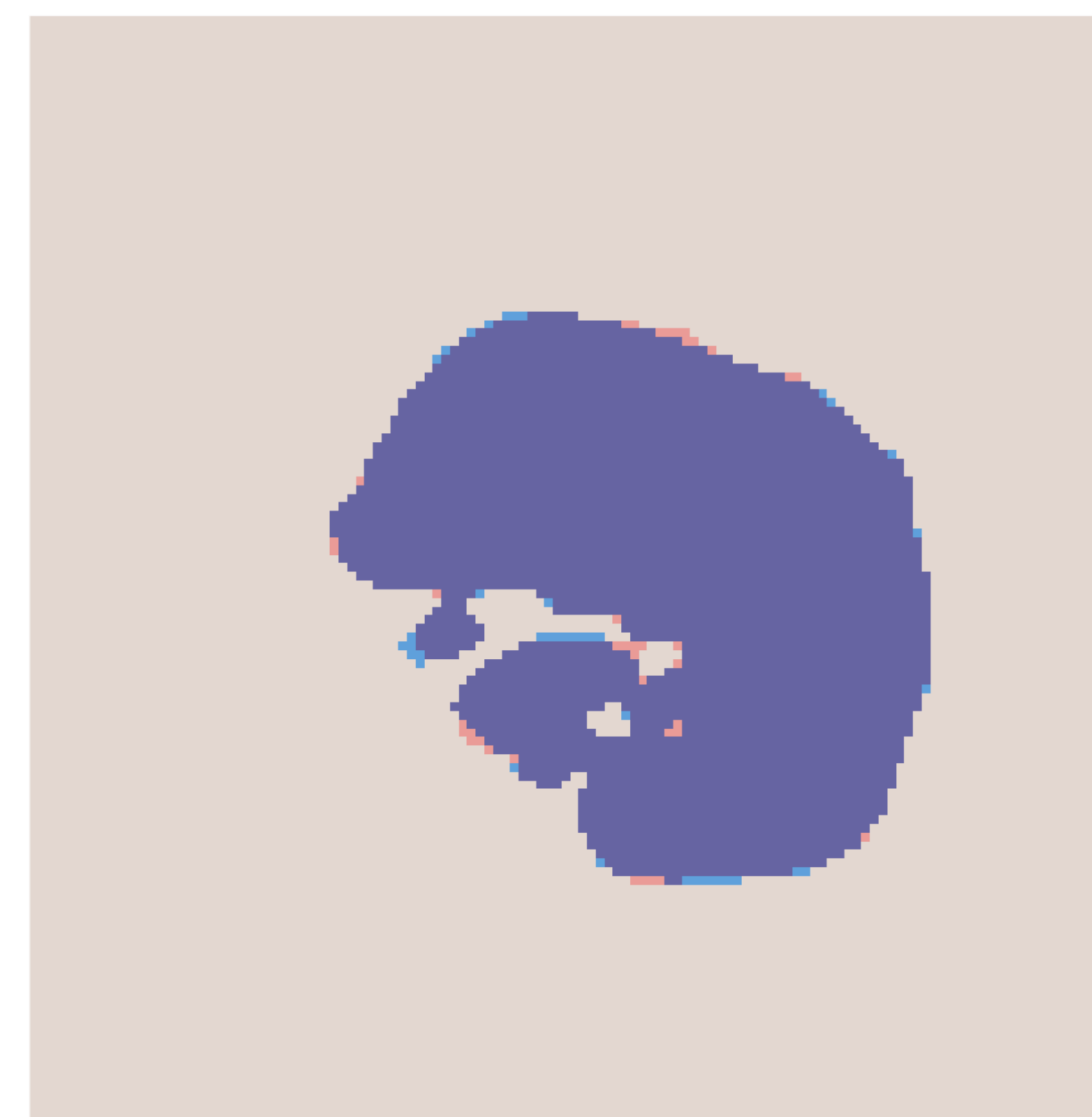
Overlapping a prediction mask (red) and a ground truth mask (blue). Left figure: the Dice loss value is 0.09 and the average energy score is -4.7. Right figure: the Dice loss value is 0.81 and the average energy score on the contour is -2.1. The Dice loss and average energy were extracted from a contextual kidney contour increased by one voxel.
