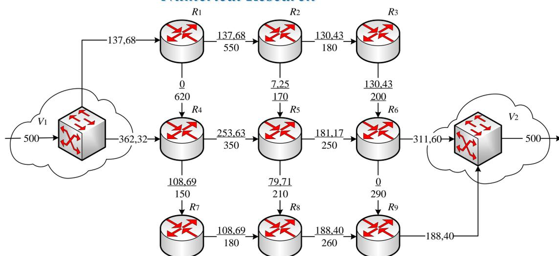
Numerical research had shown that when load balancing was implemented both at the access and network levels, the network was able to service even the flow of packets with maximum intensity. Figure shows the order of load balancing at the access and network levels at 500 1/s. The packet flow received from the first access network was balanced between the first and fourth routers in the proportion of 27.5 by 72.5%.
